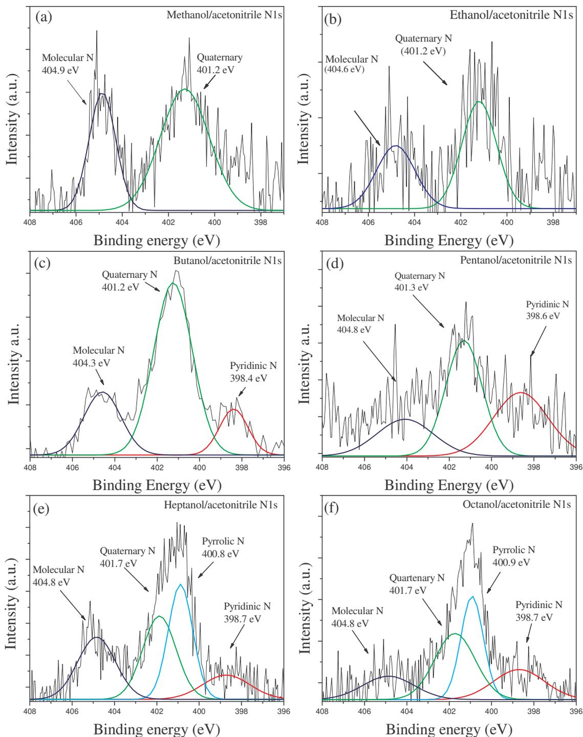
Figure 2. XPS N1s spectra of N-CNTs produced in CVD at 850 °C showing different types of nitrogen incorporated in N-CNTs when (a) methanol, (b) ethanol, (c) butanol, (d) pentanol, (e) heptanol, and (f) octanol were used in the precursor.
