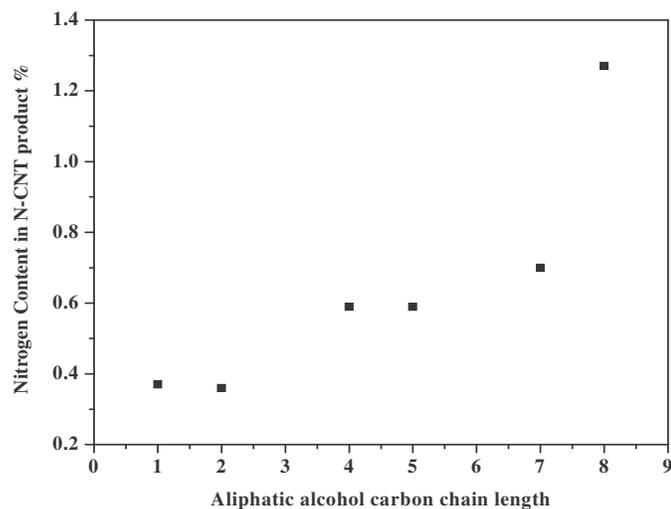
Figure 1. The N composition in N-CNTs made from the different alcohol precursor mixtures obtained from XPS analysis.
